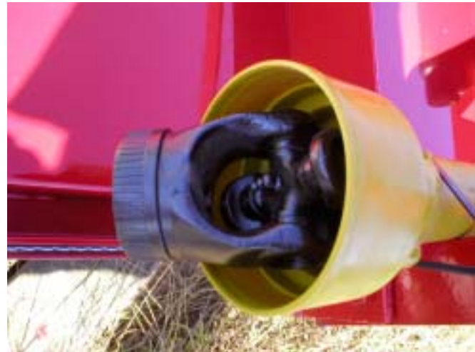
Lubricating Driveshaft Slip Joints
