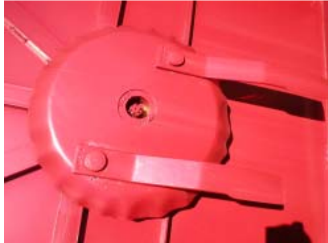
Removing Blade Holder Nut
