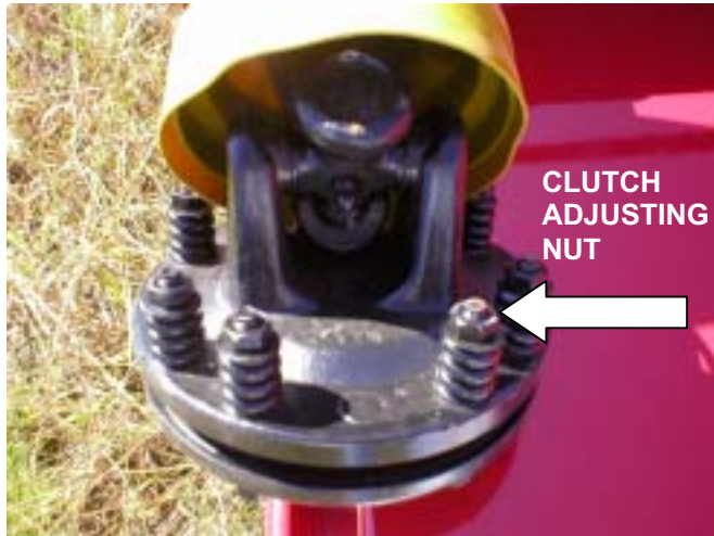
Adjusting Slip Clutch
