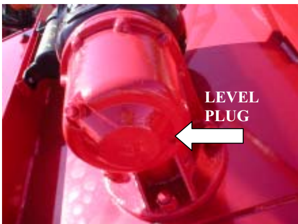
Checking Gearbox Lubricant Level
