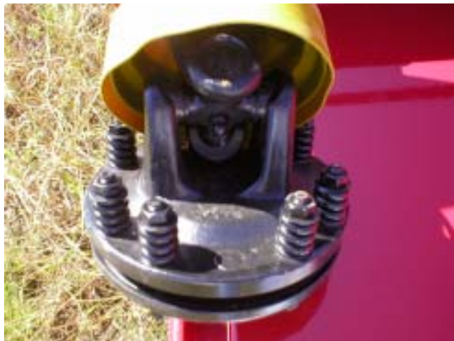
Lubricating Universal Joints
