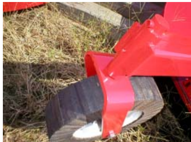
Lubricating Tail Wheel Pivot.
