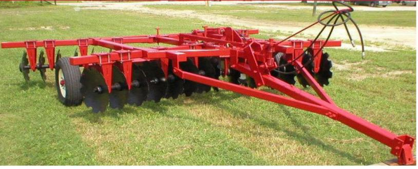
Disc Harrows are designed with durable and rigid 3 ½" tubular frames holding gangs firmly in place. Wide range of cutting angles easily adjusted for maximum protection. "Clevis" type hitch placed low for easy handling. Cutout disc blades located on front and rear. Hydraulic cylinder used to raise and lower transport wheel. 9.5L tires and tubes. Axle bearings are sealed for long life protection.
