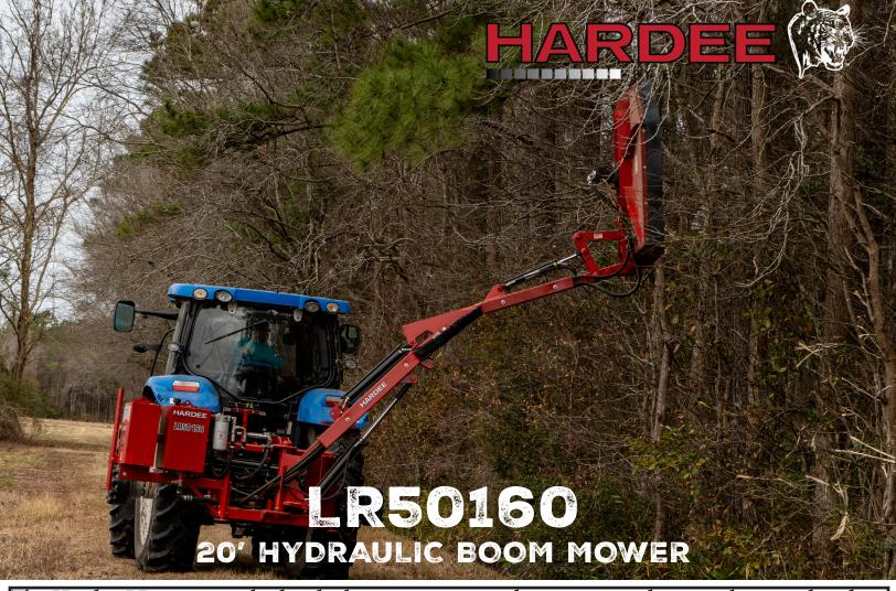
The Hardee LR50160 is a hydraulic boom mowers with a 4-axis single joystick control and proportional control valves for fine metering. It features vertical and horizontal breakaway hydraulic valves with no-drift load holding capabilities. The LR50160 is compatible with Cat. 2 & 3 3-point hitches and quick hitch spacing.
