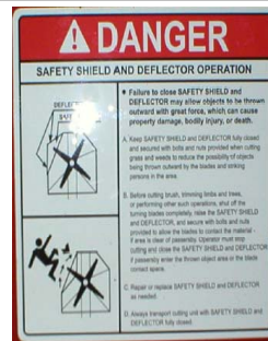
Danger – Exposed Blades (P/N – 15338)
