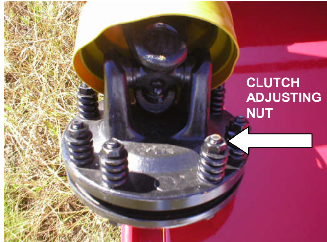
Adjusting Slip Clutch
