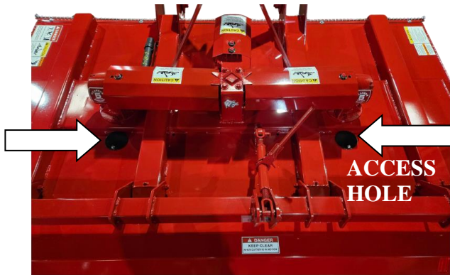
Checking Blade Bolts
