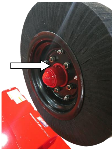
Lubricating Tail Wheel Bearings
