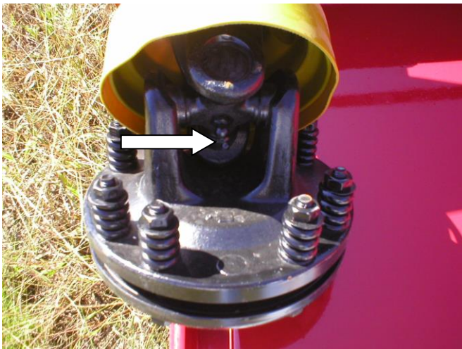
Lubricating Universal Joints
