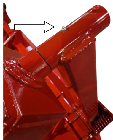
Lubricating Tail Wheel Pivot
